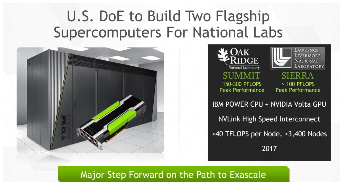
Figure 1: Summit and Sierra supercomputers at a glance. The two systems share the same system and node architecture based on GPU-accelerated OpenPOWER platform.
